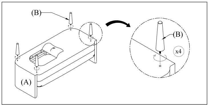
Align Leg (B) with the corresponding pre-threaded holes on the bottom of Seat (A) as shown. Screw legs in clockwise until they are secure.
